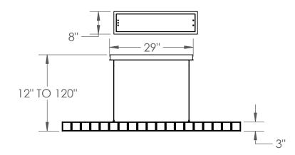
Electrical: Integrated LED Electrical Type: LED Wattage: 46 Voltage: 120 Source Lumens: 5187 Down Light: N/A Dimming: TRIAC CCT: 3000K CRI: 90 Mounting: Building Structure Weight: 185 Ibs. Suspension: Cable UL Location: Dry Slope: Flat Mount Only
